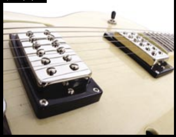
■ The TV Classics have two rows of adjustable polepieces
