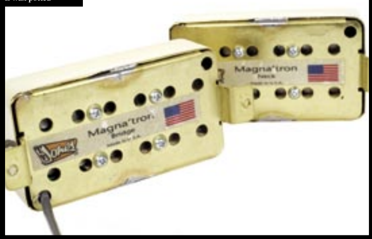
■ Soldered covers then the whole thing is wax-potted
